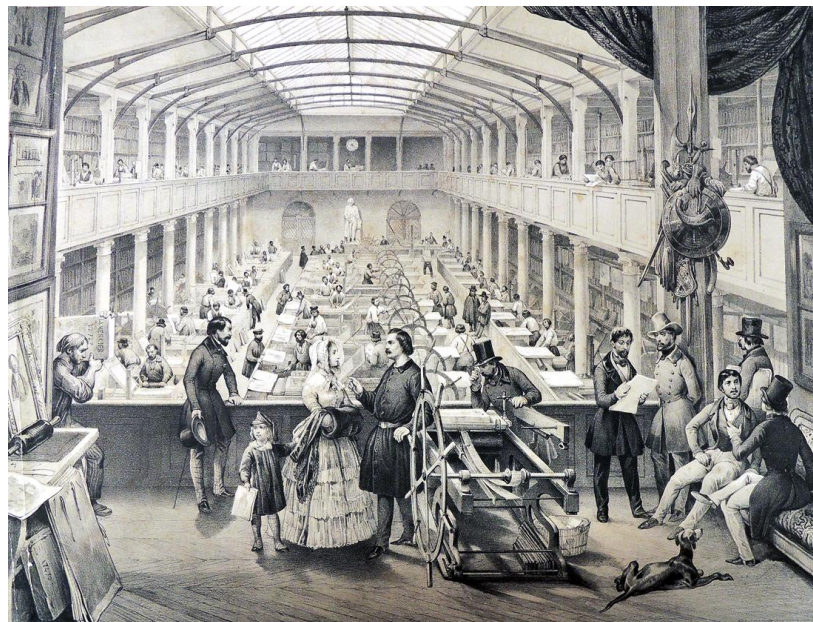
Figure 10: The lithographic printing establishment of Lemer cier & Cie., Paris, mid-1840s. In the centre, talking to a client, is Joseph Lemer cier (1803-1887) the director of the firm. Behind him on the main floor are at least thirty lithographic presses, while artists and writers work on the balconies along the sides. Against the walls are cabinets filled with hundreds of limestones, catalogued and held for reprinting. The statue of Senefelder stands at the end of the press room. [Graphic Arts Collection of the Firestone Library, Princeton GC 077]
