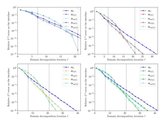
Fig. 8. Relative  $L^{\infty}$ -error computed with two-sided continuous, discrete-time (optimized at iteration  $\ell=7$  and 21) and numerical optimal (at iteration  $\ell=7$  and 21) Robin parameters, for N=20 (top left), N=50 (top right), N=100 (bottom left), N=200 (bottom right). Note the scale change for the top left figure, as explained in Figure 4. Note that, for N=20, since  $\bar{\alpha}_{D[21]}$  and  $\bar{\alpha}_{opt[21]}$  are equal, the associated curves are superimposed.
