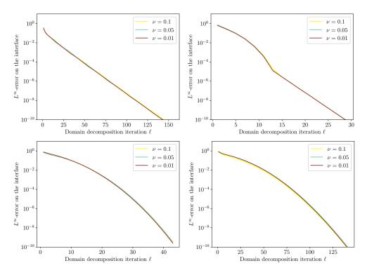
Fig. 1. Illustration of convergence, which only depends on  $\bar{\alpha}$ , for a fixed  $N:L^{\infty}$ -error, with N=100 and different values of  $\nu$ , for  $\bar{\alpha}=0.1$  (top left),  $\bar{\alpha}=0.5$  (top right),  $\bar{\alpha}=1$  (bottom left),  $\bar{\alpha}=3$  (bottom right).
